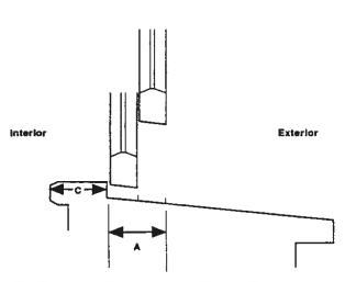
View 1. Side view of window (with no storm window) showing window trough area, A. Trough is strip across window sill where interior window sashes (on double-hung window) can touch the sill. The interior window sill (also referred to as window stool) is shown as area C.
