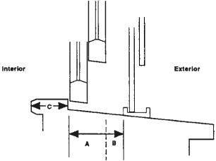
View 2. Side view of window (including storm window) showing window trough area, areas A and B. Trough extends out to storm window frame. The interior window sill (also referred to as window stool) is shown as area C.
