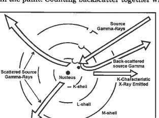
Figure 5-6. Scattering of the source gamma rays
