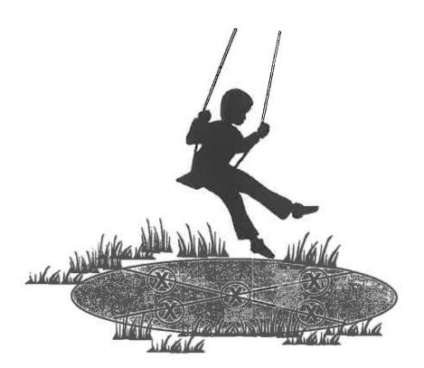
Bare soil should be divided by an x-shaped grid. Subsamples should then be collected at equidistant points along each axis.
