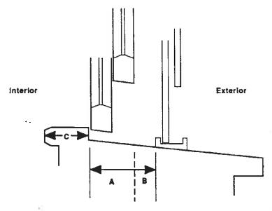
Side view of window (including storm window) showing window trough area, A and B, to be tested. Trough extends out to storm window frame. The interior window sill is shown as area C. Interior window sills and window troughs should be sampled separately.
