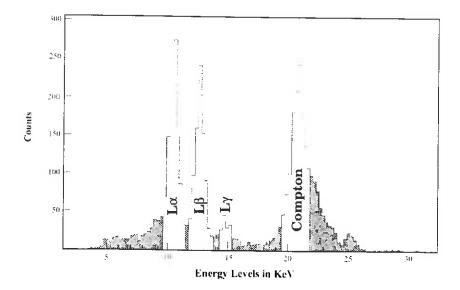
A direct reading XRF displays only the lead level.
