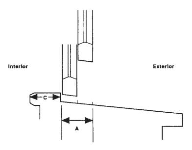
Side view of window (with no storm window) showing window trough area, A, to be tested. Trough is strip across
