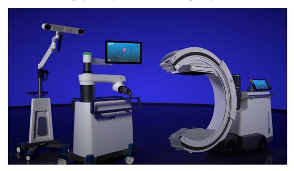
The Globus system is used to more precisely place medical devices that stabilize the spine, e.g., medical screws and rods. The system is comprised of an innovative intraoperative imaging device that can perform the functions of fluoroscopy and CT scanning, along with a robotic arm that is guided by the imaging system.
